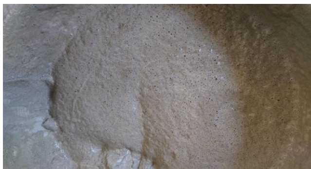
Fig.2.3.2 Freshly prepared foamed concrete mix.
