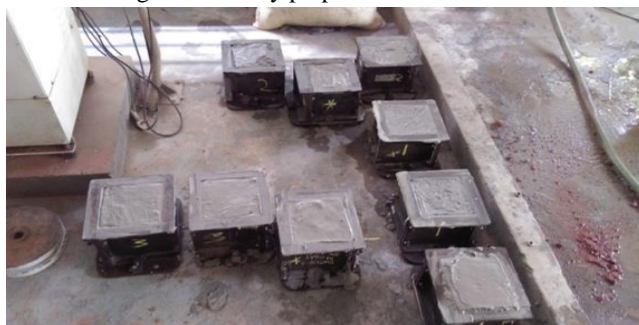
Fig.2.3.3 Foamed concrete poured in to mould
